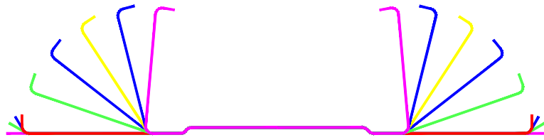
FLOWER DIAGRAM - 140 MM STRIP WIDTH, 240 MM ROLL WIDTH.
